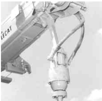
Earth boring auger on utility truck compensates movement in all planes by using "9SS" Series swivel.
